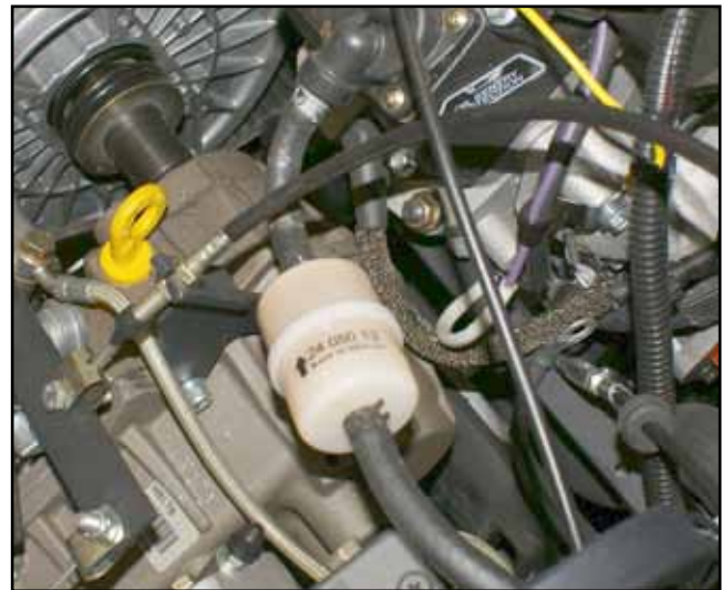
Figure 6-6a. Avenger 700 fuel filter location.
