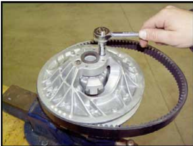
Figure 7-2a. Loosen jam nuts.
