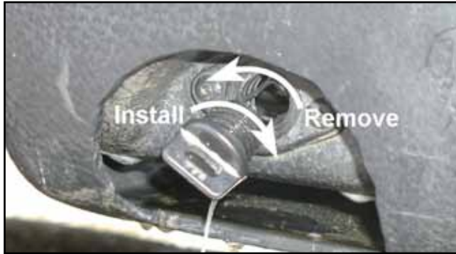
Figure 5-2. Removing and Installing the drain plug.
