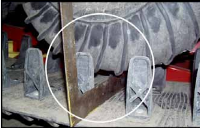
Figure 11-14. Measuring the gap of the mid tires - Frontier.
