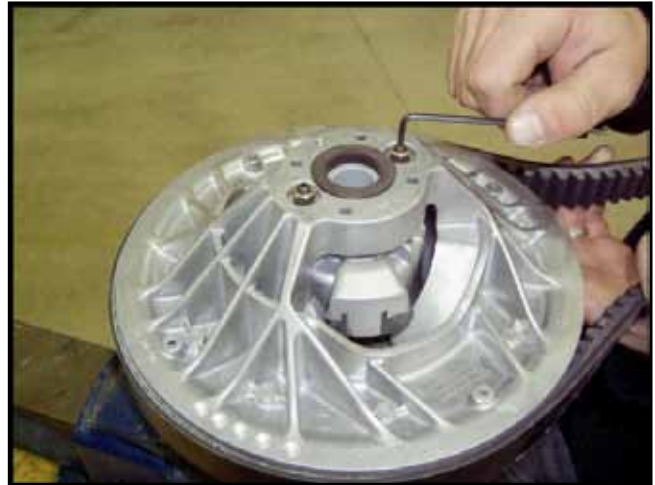
Figure 7-2b. Turn the adjustment set screw.
