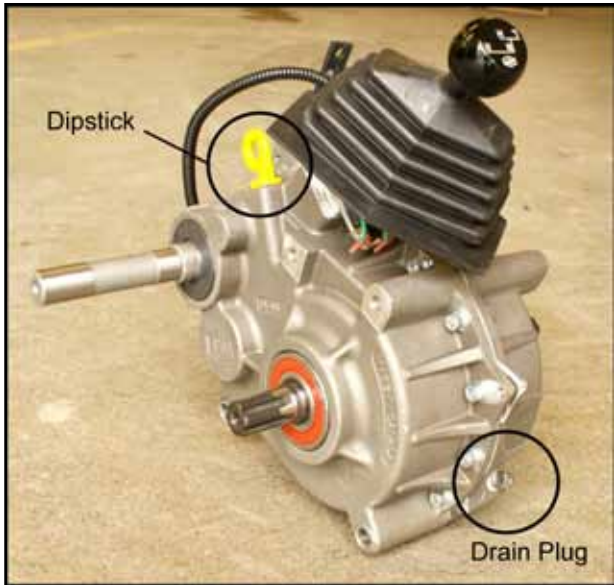
Figure 6-4a. 34-100 Transmission showing dipstick and drain plug locations
