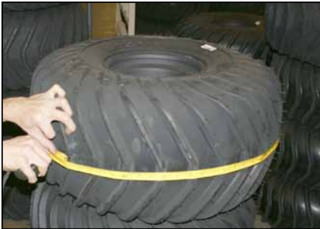
Figure 11-5. Measuring the tire.
