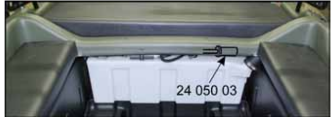
Figure 6-6. HDi and Avenger EFI fuel filter location.
