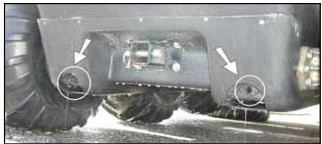
Figure 5-1. Location of rear drain plugs.
