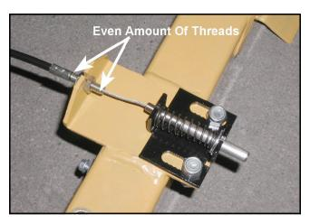
Figure 7-20. Positioning of cable at bracket.
