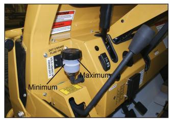
Figure 7-15. Remote translucent master cylinder well.
