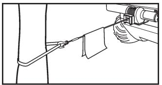
Figure 11-11. Using a cloth damper.
