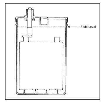
Figure 7-1. Battery Fluid Level
