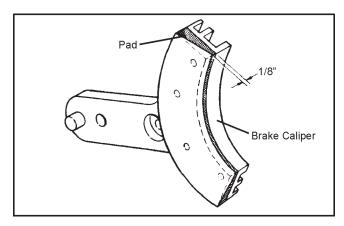
Figure 7-14. Measuring the distance between the brake disc and brake pad.
