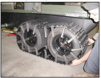
Figure 11-3. Positioning on wheel hubes.
