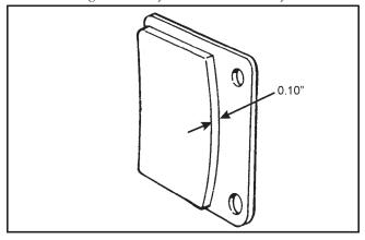
Figure 7-17. Brake pad wear, hydraulic brakes.
