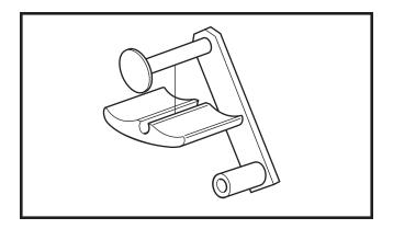
Figure 7-7. Chain tensioner components.
