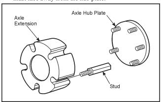
Figure 11-5. Installing the Axle Extensions.
