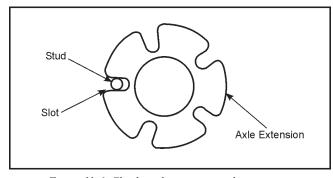
Figure 11-6. Check stud position in axle extension.
