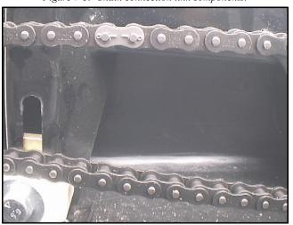
Figure 7-6. Installing the connecting link.
