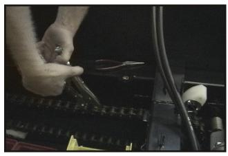
Figure 7-4. Holding chain together to insert connecting link
