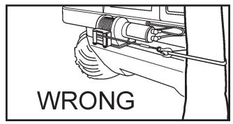
Figure 11-12. Incorrect positioning for continuous pulls.
