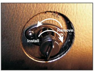
Figure 5-2. Removing and installing the drain plugs.
