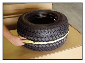
Figure 11-1. Measuring the tire.
