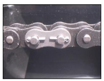
Figure 7-5. Chain connection link components.
