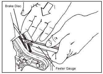
Figure 7-13. Brake pad wear, mechanical brakes.
