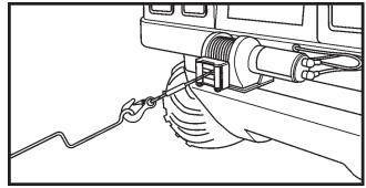
Figure 11-8. Using the Handsaver Bar.
