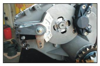
Figure 7-11. Mechanical parking/emergency brake
