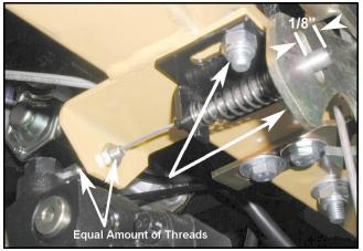
Figure 7-19. Adjusting the spring pin end of the cable.
