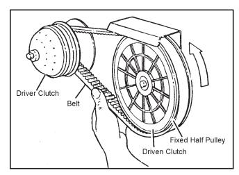
Figure 7-2. Removing the drive belt
