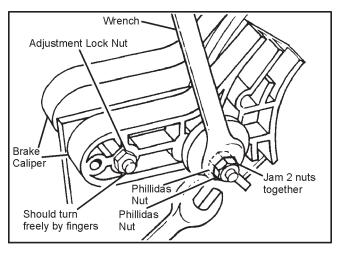
Figure 7-12. Tightening the lock nut.
