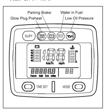
Figure 2-1. LCD Instrument Cluster.
