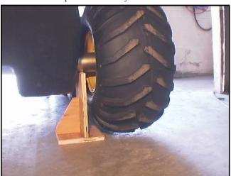
Figure 9-1. Correct placement of blocks
