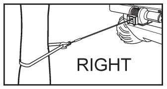
Figure 11-13. Correct positioning for continuous pulls.
