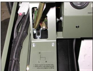
Figure 3-2. Direction of gearshift travel and gear positions.
