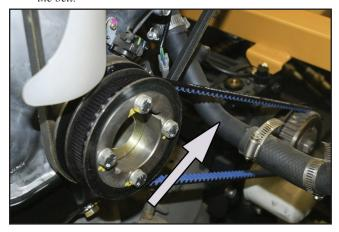
Figure 7-21. Positioning of the lower rad hose.
