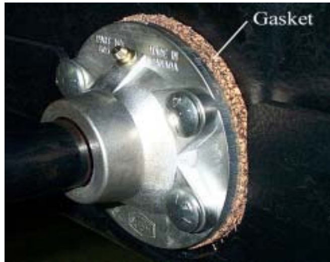
Figure 7-18. Bearing Flange and Cork Gasket
